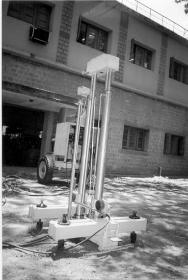
Figure 7a Cone penetrometer system
