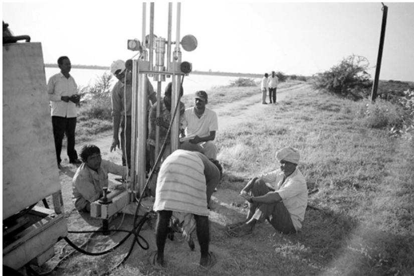
Figure 7c CPT test in progress
